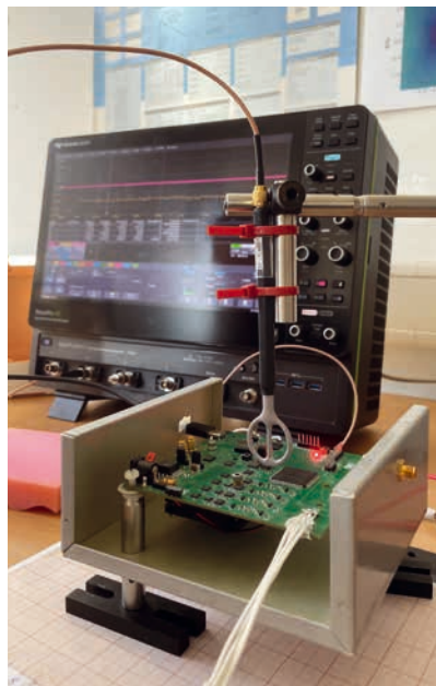
Measurement of electromagnetic emissions from a QKD component.
